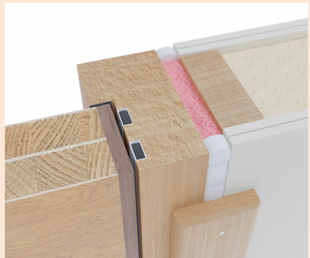
Image B – FD90 & FD120 foam with intumescent & acoustic acrylic sealant cap of 10mm minimum.
